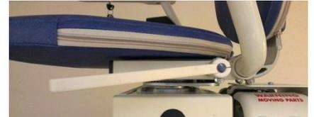
To return the seat to the normal travel position, lift one of the seat swivel levers (3) and swivel away from the landing until the seat comes to a stop then release the lever to lock the seat in place.
